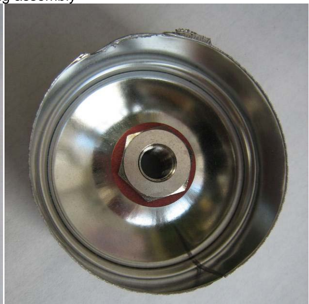
Inside view of the screw fitting mounted on the bottom of the container
