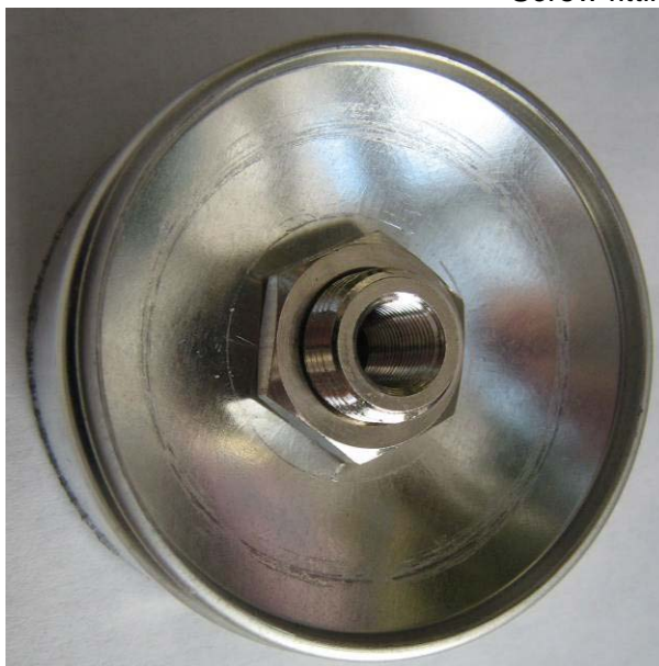
Outside view of the screw fitting mounted on the bottom of the container
